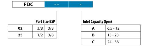
Ordering Code Example: FDC25B - 1/2 - 3/8 BSP Ported Manifold, 13/23 lpm Inlet Range Capacity.
